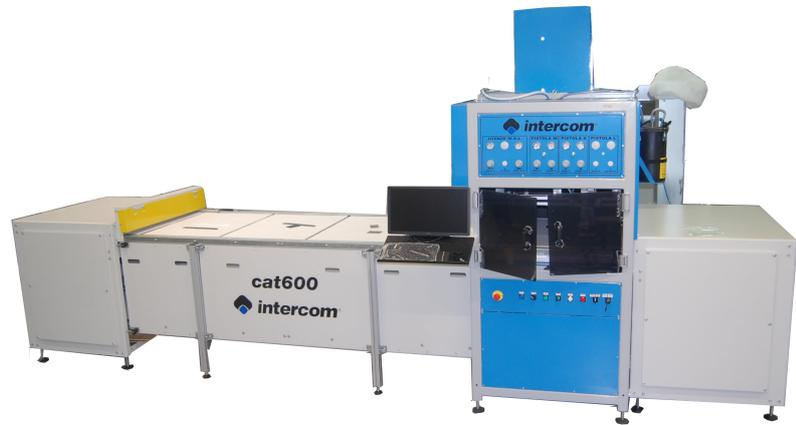
Automatic moving of the pallets: in this configuration are included a minimum of 16 pallets mm 850x615. This configuration allows the operator to have always at his disposal 4 pallets in front of him where to place the materials and then take them back for the coupling phase.
